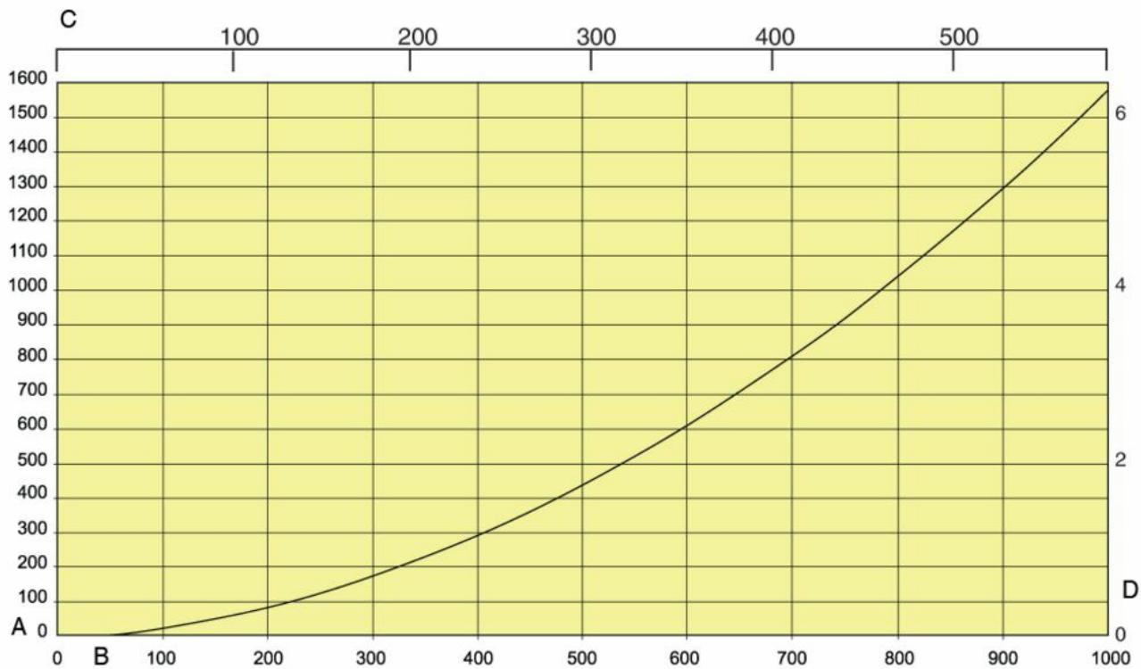
A: Pressure drop (Pa) B: Airflow (m<sup>3</sup>/h) C: Airflow (cfm) D: Pressure drop (in. w.c.) Pressure drop valid for 6 and 7m track with 5 m hose Ø125mm and HB 600LL nozzle Airflow recommendations: Heavy vehicles: 1000 - 1200 m<sup>3</sup>/h Car / SUV: 400 - 600 m<sup>3</sup>/h
